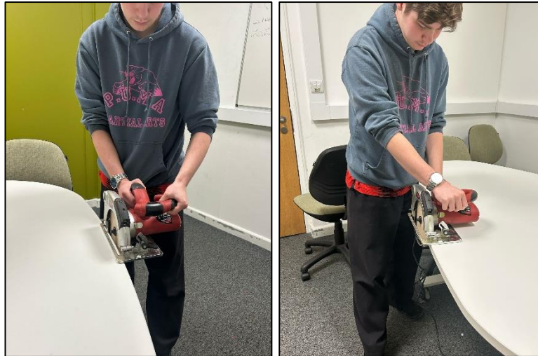
Figure 2: In-depth Circular Saw Interview participant mimicking use of the saw during the interview. LEFT: The participant holds the saw with the blade oriented away from them. RIGHT: The participant holds the saw with the blade oriented towards them.
