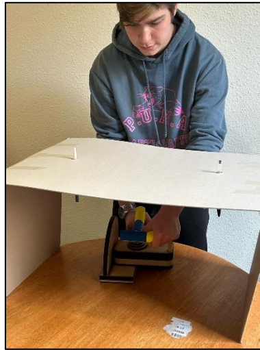
Figure 9: Participant completing Texture Influence Test. They are gripping the test piece with varying textures applied under a cardboard platform to block their view while allowing sufficient space to mimic the operation of the tool.
