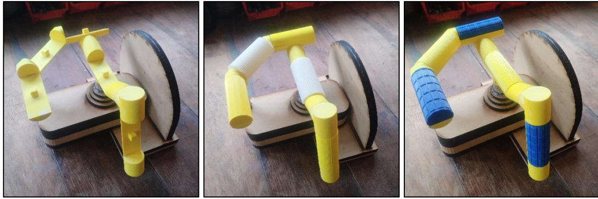
Figure 8: LEFT: Empty base Test Piece. MIDDLE: Smooth grips on areas 1, 4, and 5 lower; and Lines grips on areas 3 and 5 upper. RIGHT: Square grips on areas 1, 4, and 5 lower; and Smooth grips on areas 3 and 5 upper.
