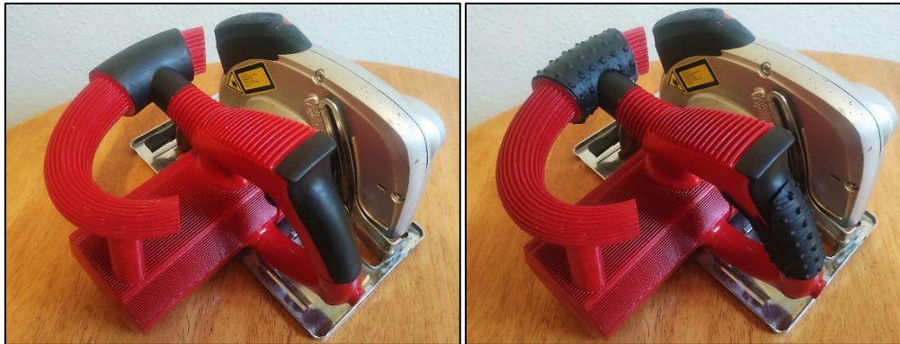
Figure 11: Prototype Colour Test Piece. LEFT: Colour test piece (Smooth and Lines textures). RIGHT: Colour test piece with DOTs applied to intended handle positions (Dots and Lines textures).
