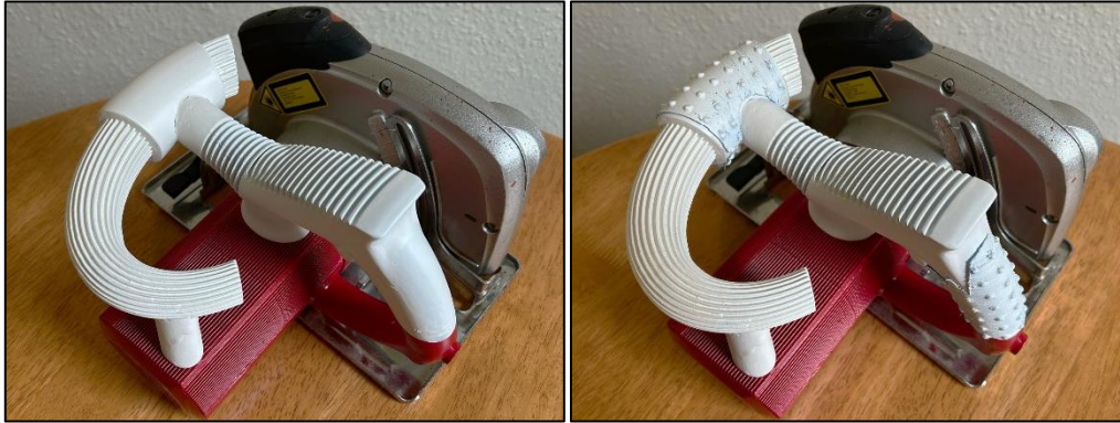
Figure 10: Prototype Monochrome Test Pieces. LEFT: Monochrome test piece (Smooth and Lines Textures). RIGHT: Monochrome test piece with DOTs applied to intended handle positions (Dots and Lines Textures).
